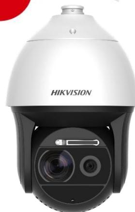
Hikvision 4K series DS-2DF8836I5V-AELW smart PTZ dome cameras are able to capture high quality images in dim light environment with its laser IR light, which can reach up to 500m IR distance. Embedded with 1/1.9" progressive scan CMOS chip makes WDR and 8MP real-time resolution possible. With the 36X optical zoom Day/Night lens, the camera offers more details over expansive areas.
