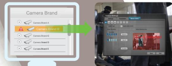
NUUO NVRsolo embedded motion detection function can work with any IP video devices which are supported by NUUO Device Pack. It helps user to minimize the installation time from toggling between camera web setting page and NUUO NVRsolo menu.
