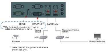
\*\* IMPORTANT: Use a network computer remotely for ongoing operations. Only connect directly to a monitor for trouble-shooting.
