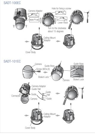
\* Conditions for Installation : The installation place should be able to bear up to 4 times of the total product weight (about 16Kg). This product is to be used when the thickness of the ceiling board is less than 40mm. This product requires a minimum of 180mm space above the ceiling board.
