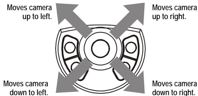
Camera movement speed is directly proportional to the distance the **Tracker Ball** moves from its center position. For example if the **Tracker Ball** moves slightly to the right, the camera pans slowly to the right. As the **Tracker Ball** moves farther to the right, the panning speed increases until maximum speed is reached.
