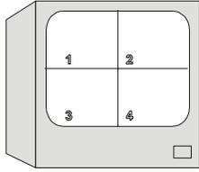
Video displays from 4 cameras when **2x2** format is active. 4-, 9-, and 16-camera multiplexers support this display format.
