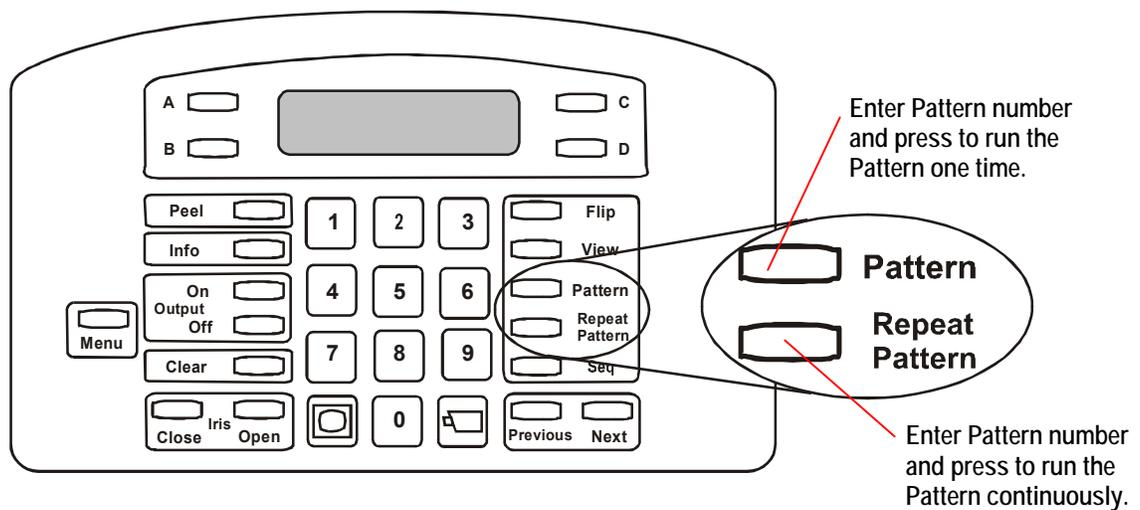
*Chapter 4* provides Pattern programming instructions. If a list has been compiled for your facility, refer to the **Programming Worksheets** (8200-0306-04) to determine which Patterns are available for the installed domes.
