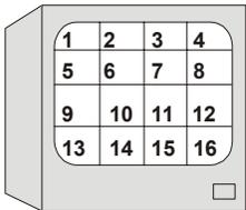
Video displays from 16 cameras when **4x4** format is active. 16-camera multiplexers support this display format.
