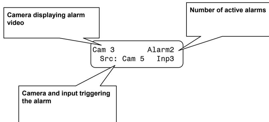
The default system setting automatically clears alarms after 60 seconds. No action is required by the operator to clear alarms as long as automatic alarm acknowledgment is enabled. However, alarms can manually cleared by pressing the **Clear** button on the Primary Controller. Figure 3-16 illustrates the location of the **Clear** button.
