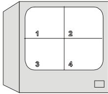
Quad display mode allows video from 4 cameras to be displayed at once on the monitor. The camera number appears in the bottom of its respective quadrant on the monitor.
