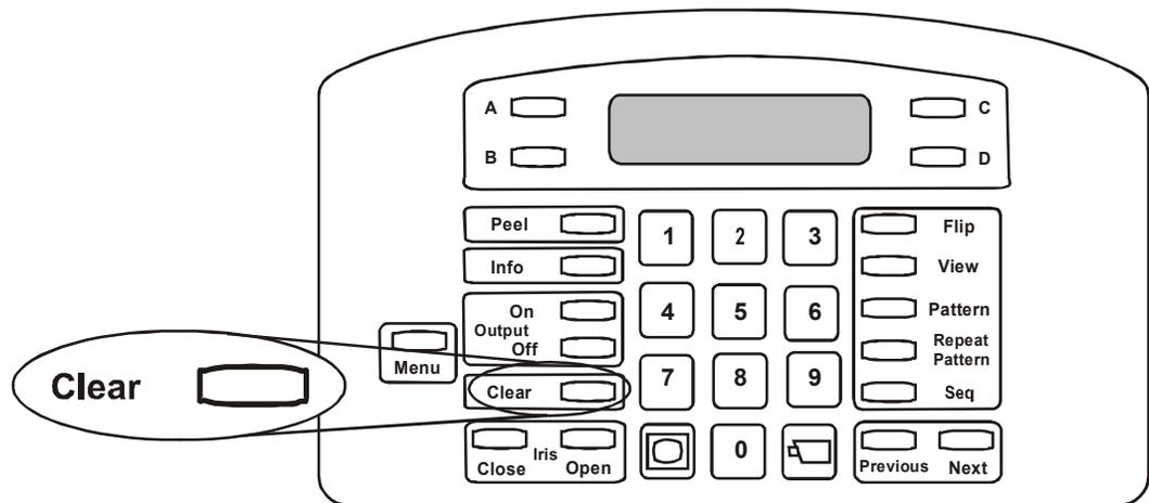
When you clear an alarm, its associated output returns to its original state, and the alarm information is removed from the LCD. Continue to press **Clear** until all active alarms have been acknowledged.
