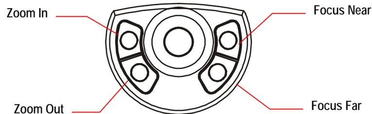
**Zoom** refers to adjusting the magnification of the camera lens to make an object appear closer (larger) or more distant (smaller). To make objects appear closer to the camera, press **Zoom In**. To make objects appear more distant from the camera, press **Zoom Out**. Quickly pressing and releasing a zoom button displays only a slight visible change on the monitor. The longer a zoom button is pressed, the more noticeable is the response.
