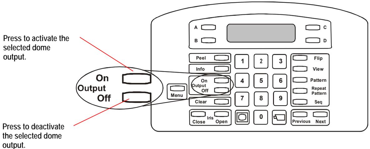
The following procedure describes how to activate or deactivate a dome output. You must know the dome number and the output number before performing this procedure.
