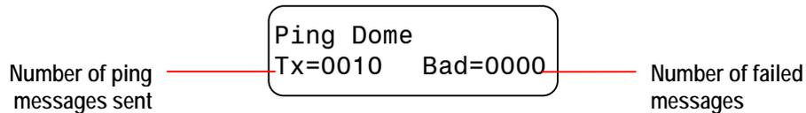
4. Press **Next** to display the controller ping test information.
