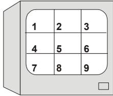
Video displays from 9 cameras when **3x3** format is active. 9- and 16-camera multiplexers support this display format.
