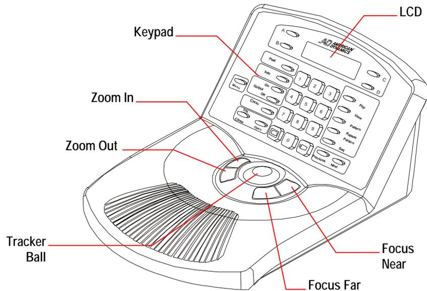
The **Tracker Ball** provides variable speed control of a camera's pan and tilt.
