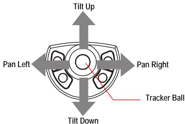
You can simultaneously pan and tilt the camera for diagonal movement. Moving the **Tracker Ball** diagonally up and to the right moves the pointing direction of the camera up and to the right. Figure 3-5 illustrates diagonal camera movement.
