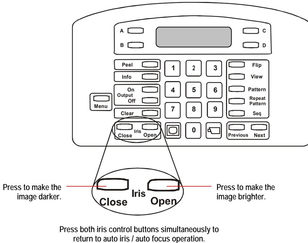
Press **Iris Close** to make the picture darker. Press **Iris Open** to make the picture brighter. To return to auto iris/auto focus mode, press both iris control buttons simultaneously.
