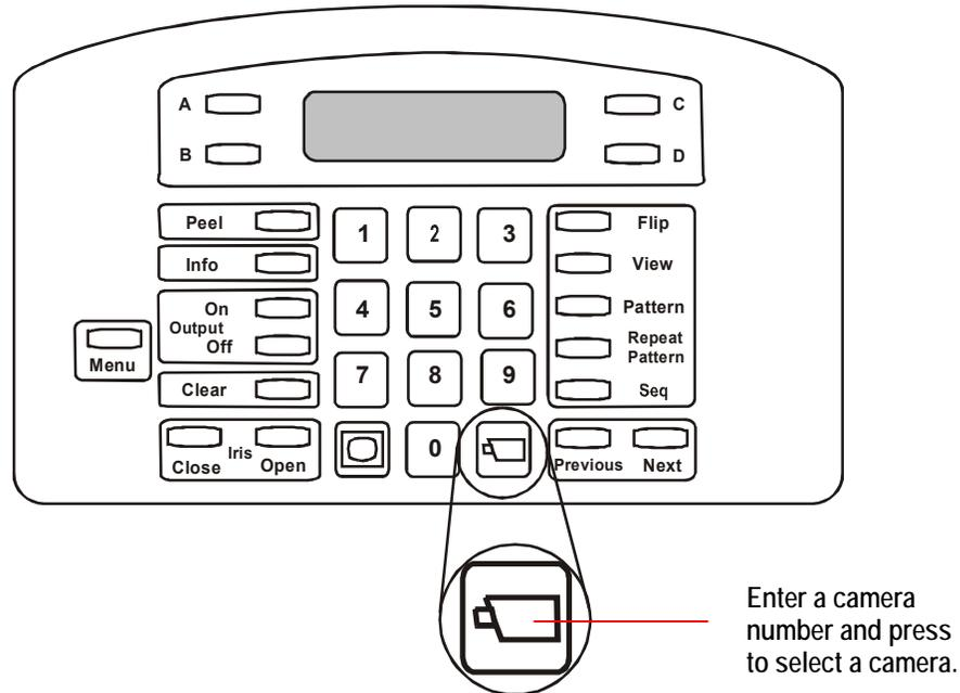
Full-screen video from the selected camera appears on the monitor. The associated camera number appears in the bottom left corner of the monitor. If the camera is selected via the Primary Controller, video appears on the Main monitor. If the camera is selected via the Secondary Controller, video appears on the Call monitor.
