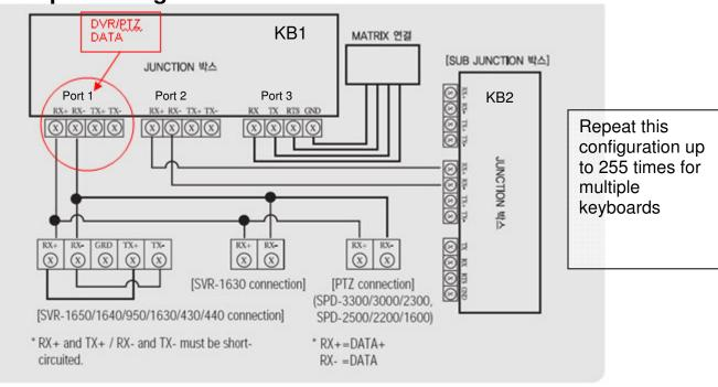
All supported SPEED DOME functions can be controlled when the PTZ camera is connected through the SVR-1650/1640/950.
