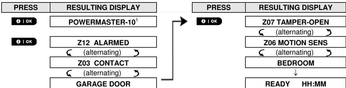
In response to additional clicking of the **OK** button, the display shows details of other events retained in *open tamper (if any), or reverts to its initial state (see A above)*.
