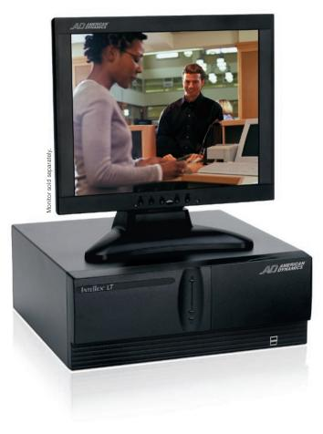
Intellex LT delivers the key Intellex features in an economical package, providing the best solution for small retail stores, health care facilities and small offices. It can store more than 900 hours of video and supports as many as five simultaneous Network Client users.
