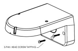
Use the mounting plate and choose the correct three screw holes.
