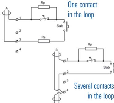
The magnetic contact MC 440 with 2 built-in resistors for a balanced circuit. When installing the magnetic contact it is easy to select if one resistor or both should be used (see wiring diagram) For quick and easy installation the magnetic contact comes with screw terminals with wire protection. It is equipped with tamper protection against unauthorized opening.
