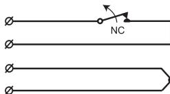
MC 255-LSZH is a universal magnetic contact in small format with NC function and halogen-free cable that can be used both in alarm and access control systems for monitoring e.g. doors and windows against unauthorized opening.
