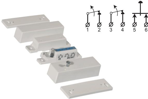
MC 447 is a surface mount magnetic contact with double NC function and 6 screw terminals. It can be used in both alarm and access control systems for monitoring e.g. doors and windows against unauthorised opening.
