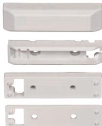
Plastic housing for surface mount installation of MC 340, 346 and 347. Contact and magnet are placed in the respective brackets. Delivered with brackets, covers and with a 6 mm and a 3 mm plastic spacer.
