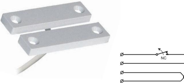
MC 740P is a small and thin magnetic contact with NC function that can be used in both alarm and access control systems for monitoring e.g. doors and windows against unauthorized opening.
