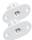
Plastic flange for installation of recessed magnetic contacts into non-magnetic door and window frames with screws. Suitable for MC 240, 246, 247, 250, 270 and 272. Contact and magnet are screwed into the adapter, which allows for adjustment of the operation gap.
