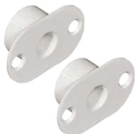
Plastic flange for installation of recessed magnetic contacts into non-magnetic door and window frames. Suitable for MC 340, 346, 347 and 370. Contact and magnet are pressed into the adapter and mounted with the included screws.
