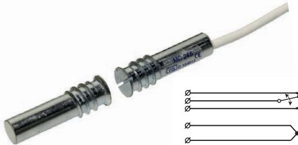
MC 246 is a universal magnetic contact with change-over (NC/NO) function that can be used in both alarm and access control systems for monitoring e.g. doors and windows against unauthorized opening.
