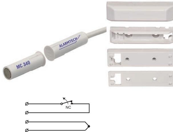
MC 340-S3 is a universal magnetic contact set with NC function that can be used in alarm and access control systems for monitoring e.g. doors and windows against unauthorized opening. Both the contact and the magnet part are in a water proof (IP 67) plastic housing.
