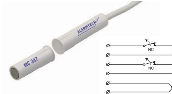
MC 347 is a universal magnetic contact with double NC function that can be used in both alarm and access control systems for monitoring e.g. doors and windows against unauthorized opening.
