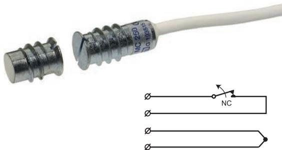
MC 250 is a universal magnetic contact in small format with NC function that can be used in both alarm and access control systems for monitoring e.g. doors and windows against unauthorized opening.
