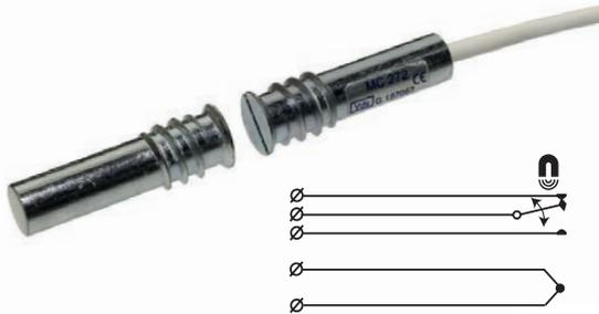
MC 272 is a universal magnetic contact with a change-over (NC/NO) function for high security systems that can be used both in alarm and access control systems for monitoring e.g. doors and windows against unauthorized opening.
