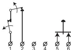
MC 470 is a surface mount high security contact with NC function with 6 screw connections and sabotage contact.
