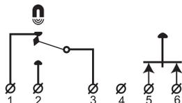
MC 472 is a surface mount high security contact with change over NC/NO function with 6 screw terminals and sabotage contact.
