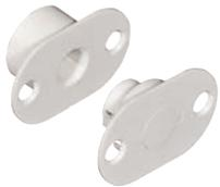
Plastic adapter with extra strong magnet for installation of recessed magnetic contacts in door and window frames of steel or in spaces where greater operation gap is required. Suitable for MC 340, 346 and 347. The contact is pressed into the adapter and mounted with the included screws.
