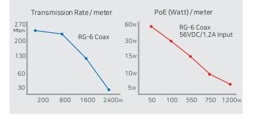
The test result was conducted using ECP-2701 as transmitter.
