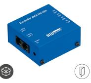
Expander 4xDI 1W-UNI Industrial 4× digital inputs on 3 m cable
