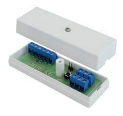
JB 370 is a junction box which simplifies the installation of the GD 370 glass break detector. The junction box connects GD 370 with IU 370 and/or multiple JB 370. JB 370 is equipped with a built-in resistor for termination of glass break (optional with jumper). It also has tamper protection.
