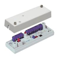
The IU 370 is an analyser and relay unit, used to connect the GD 330 and GD 370 glass break detectors to a control panel. Up to 10 detectors can be connected to the device.
