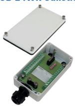
JB 24WH is a 24 terminal junction box in metal designed for use outside or in cold environments. It is equipped with an internal heating element and tamper switch. The junction box is intended for alarm and access control systems where a more durable and safe box is needed. The cable entry is made of UV resistant plastic and allows for a cable diameter of 4.5–10 mm.
