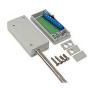
The JB 50 is a 10-terminal junction box in metal with tamper switch for connection of seismic detectors, where increased safety and durability is required. The box has 10 screw terminals with wire protection, 2 of which are specified for the tamper switch. The box has an input for the stainless steel hose MC T2, T4 or T7, which locks with grooves inside the box for safe installation and operation. The box is easy to mount with screws.
