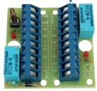
The RC 020 is a relay card with two relays and dual (2x) alternating (NC/NO) functions. Connection is provided via screw terminal with wire protection. Active relays are indicated by LED. The card also has an anti-tamper switch to protect against unauthorised opening if the card is installed, for example, in a JB 200 box.
