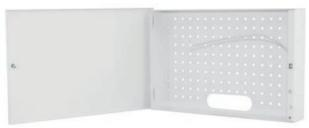
JB 400 is an empty metal housing with tamper protection against forced opening. Suitable for external equipment such as relay cards and terminal blocks. There are pre-drilled holes at the back of the housing for installation of enclosed plastic spacers.
