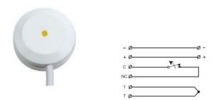
The GD 370 is a glass break detector with relay output that can be directly connected to a control panel. It is especially designed for monitoring of laminated glass panes but is also suitable for standard window glass.
