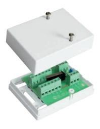
JB 370-2 is a junction box which simplifies the installation of the GD 370 glass break detector. The junction box connects max 2 GD 370 with IU 370 and/or multiple JB 370/JB 370-2/JB 370-5. JB 370-2 is equipped with a built-in resistor for termination of glass break (optional with jumper). It also has tamper protection.
