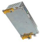
Power supply unit as a module for DIN-rail mounting with ViP (Voltage in Parallel) function, 24 VDC 6.5 A.
