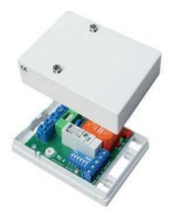
RC 230 enables control of a high voltage load up to 2000 VA with a magnetic contact or low voltage detector. It has a built-in programmable timer function for ON or OFF control. The time is programmed with a DIP-switch, from 0 s to 16 hours. The high voltage relay has a changeover function that can switch 250 V AC max 8 A. The relay circuit is protected by a 10 A fuse.
