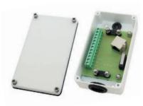
JB RJ45 is a junction box with a RJ45 jack and 12 terminals, 2 of which are intended for the tamper switch. The junction box is intended for alarm and access control systems where a more durable and safe box is needed. There are 3 cable entries, at the top, bottom and back, for discreet installation. The box is also equipped with strain relief for the RJ45 connector. The screw terminals feature rising cage clamp for secure installation.
