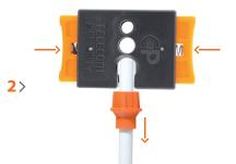
Insert the coaxial cable into the side slot of the stripping tool (SPC) about 10 mm (3/8"); gently squeeze the blades while pulling the cable out to slit both sides of the jacket.
