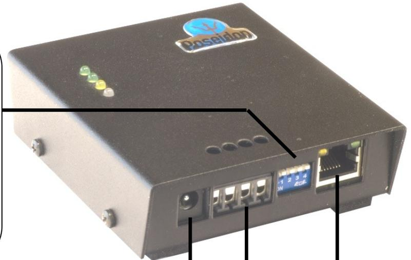
**1.2)** Plug the power adapter to a mains outlet (230 / 110V) and connect it to the Poseidon 12V power connector.
